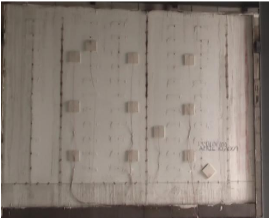
Figure 7 Unexposed side after the application of hose stream on the exposed side, no visible failure and comparable to Figure 2 At 00:00:00
