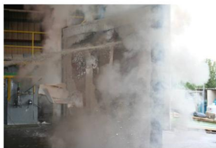
Figure B-9. Application of Hose Stream Test.
